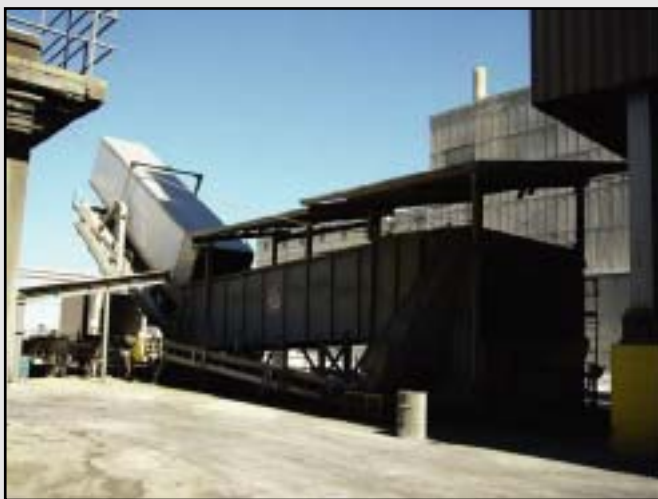
Scrap Tires remain on trailers until they are ready for use. Shown above, a trailer being tipped to remove tires.
