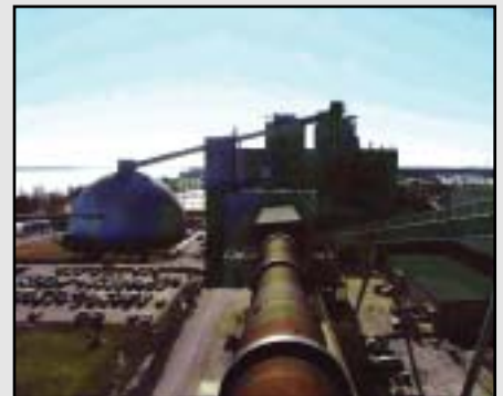
View of kiln showing approximate mid-kiln location of scrap tire injection point.
