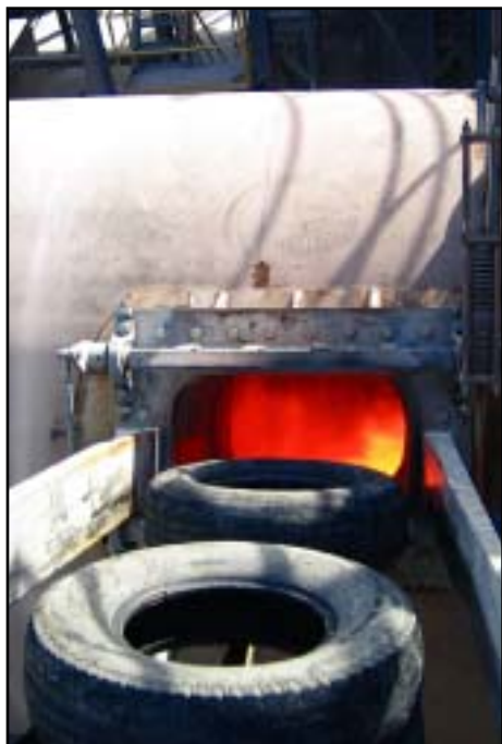
Scrap tire being introduced into kiln.
